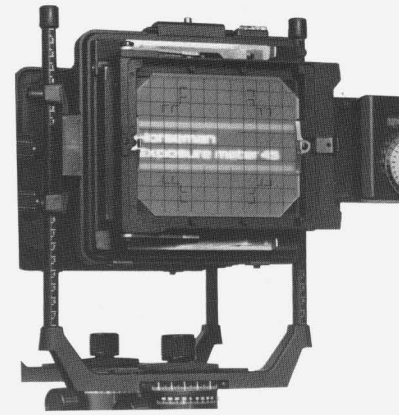
The probe for this film plane exposure meter can be placed anywhere on the ground-glass image. Because it reads the light coming through the lens, it automatically compensates for the lens extension and any filters that are used.
