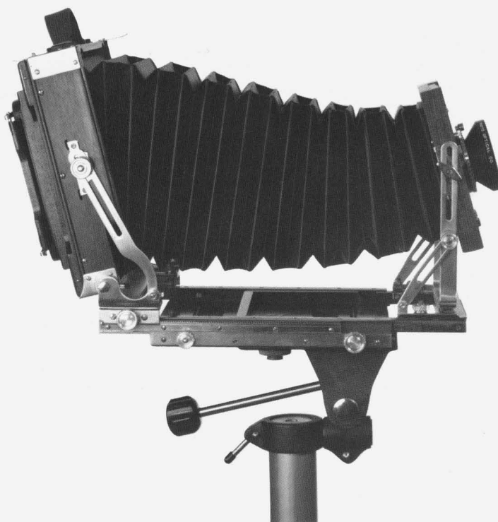
The back section of this camera pivots from a base axis (for tilts) and the lens-board frame pivots at the axis of the lens.
