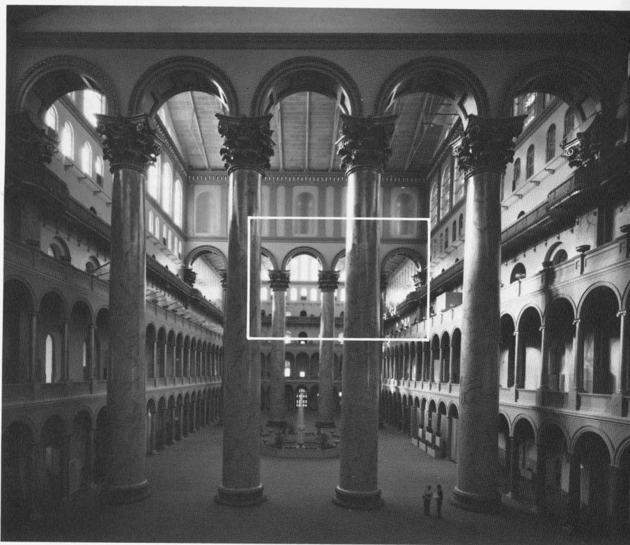
Angle of view changes with film format. The outer area of the picture represents the angle of view with a 4 x 5 camera using a normal lens. The inner area represents the much smaller view obtained if the same lens focal length is used on a 35 mm camera.
