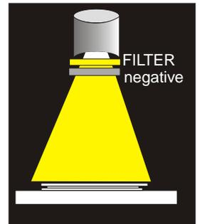
It is better to place the filter above the negative than in the holder below the lens which might distort the image.
